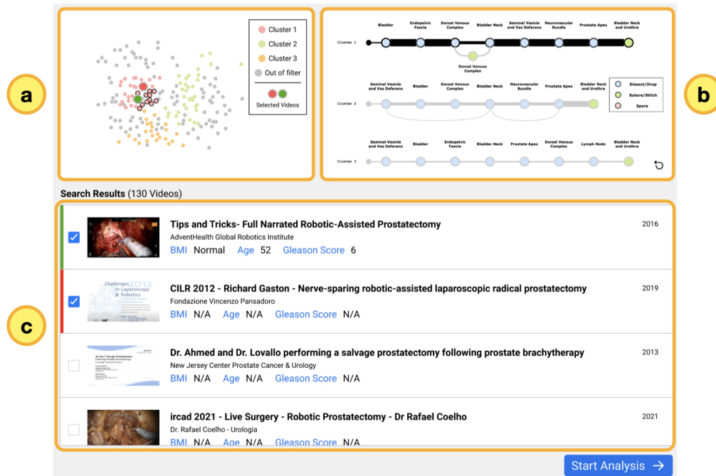
Fig. 1. Users can search videos based on semantic and structural information of procedures using our prototype's video search UI. (a) Clustering Visualization: clustering results of surgical procedures are displayed, in which a dot represents a video clip. (b) Procedural Diagram: users can see the overall structure of procedures and filter the videos by clicking the nodes or edges of a diagram. (c) Filtered Video List: users can see a list of videos that are filtered by the procedural diagram.
